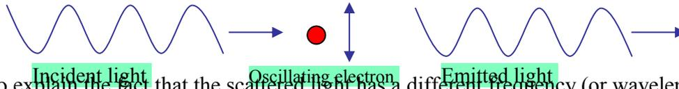
To explain the fact that the scattered light has a different frequency (or wavelength), Compton said that the scattering is a collision between particles of light and electrons. But we know that momentum and energy is conserved in scattering between particles. Specifically, from conservation of energy  $h\nu + m_e c^2 = h\nu' + (p_e^2 c^2 + m_e^2 c^4)^{1/2}$ . The last term is the energy of the scattered electron with mass  $m_e$ . Next, use the conservation
