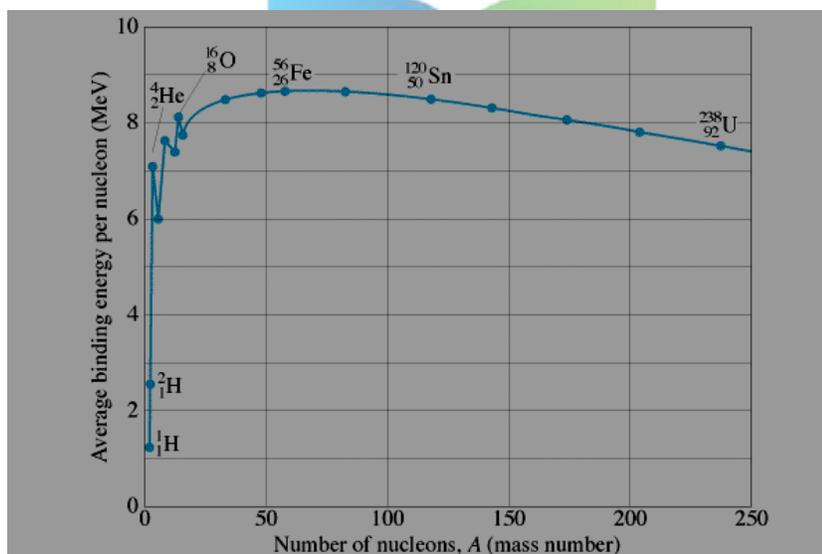
can see from the graph below, the most stable element is iron,  $^{56}\text{Fe}$  with a BE per nucleon of about 8.6 MeV. This is why iron is the heavy element found in the largest quantity on earth and inside stars. The curve is not smooth and you see that a  $^4\text{He}$  nucleus (i.e. an  $\alpha$  particle, has a relatively high binding energy and so is relatively stable. In contrast, Uranium  $^{235}\text{U}$  or deuterium  $^2\text{H}$  are much less bound and they decay.
