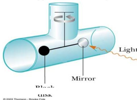
Thus the momentum of the light changes and this creates a force that rotates the mirror. The force is quite small - just  $5 \times 10^{-6}$  Newtons per unit area (in  $\text{metre}^2$ ) of the mirror.
