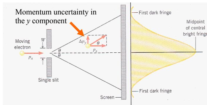
Thus we have found that  $\Delta p_y \Delta y \approx \hbar$ . The important point here is that by localizing the  $y$  position of the electron to the width of the slit, we have forced the electron to acquire a momentum in the  $y$  direction whose uncertainty is  $\Delta p_y$ .
