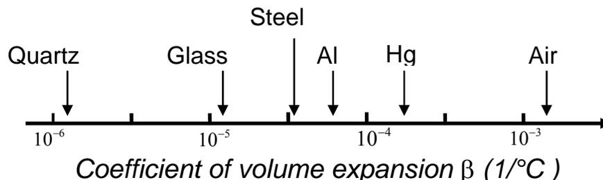
13. We can use the fact that different metals expand at different rates to make thermostats. For example, you need a thermostat to prevent an electric iron from getting too hot or a
