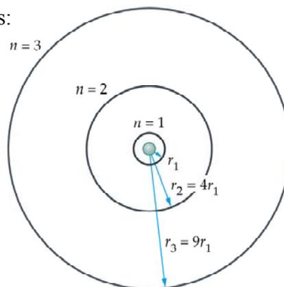
14. In the Bohr model, electrons can jump between different orbits due to the absorption or emission of photons. Dark lines in the absorption spectra are due to photons being absorbed, and bright lines in the emission spectra are due to photons being emitted. The energy of the emitted or absorbed photon is equal to the difference of the initial and final energy levels,  $h\nu = E_f - E_i$ . The picture below shows the electron in the  $n = 7$  and
