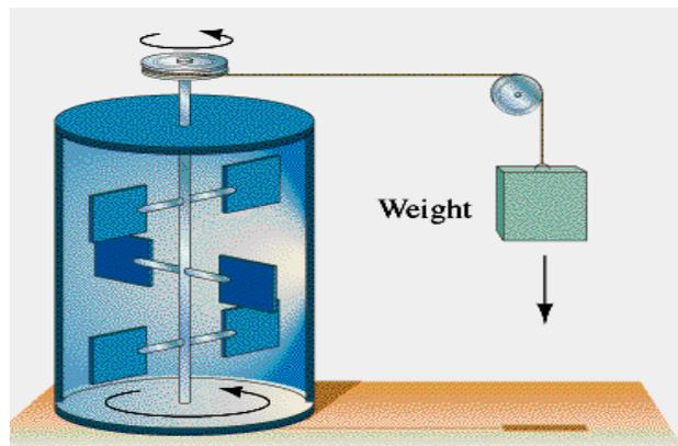
Joule established the units for the mechanical equivalent of heat. The units we use today are:
