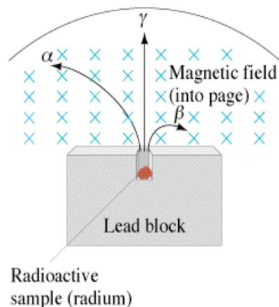
a) Heavy positively charged particles are bent to one side by the magnetic field. The amount of bending shows that they are  $\alpha$  particles.
