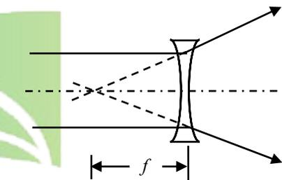
12. Here is how a concave (or divergent) lens forms an image. An observer on the side opposite to the object will see the image upright and smaller in size than the object.
