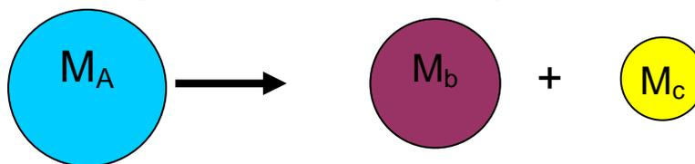
The masses of the two nuclei add up to less than the mass of the parent nucleus, and the energy released is  $Q = (M_A - M_b - M_c)c^2$ . This goes into kinetic energy and sends the two daughter nuclei flying apart at a large velocity. There happen to be NO completely stable nuclei above  $Z = 82$ , and no naturally occurring nuclei above  $Z = 92$ . Above these limits the nuclei decay or fall apart in some fashion to get below these limits.
