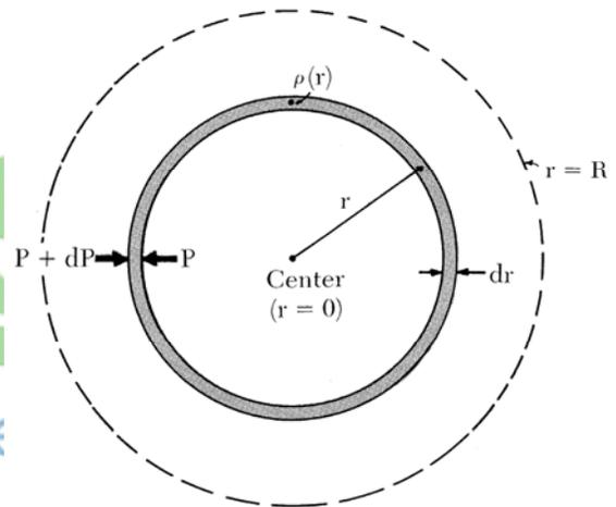
Look at the second diagram. Let  $M(r)$  be the mass contained within radius  $r$ . We will not assume that the density is constant in  $r$ . First find the inward directed gravitational force on a shell of matter at radius  $r$  and thickness  $dr$ ,  $dF = -\frac{GM(r) \times \rho(r) 4\pi r^2 dr}{r^2}$ . There is a
