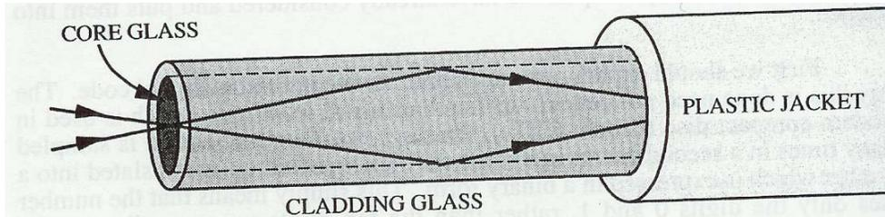
Even if the cable is bent, the light will continue to travel along it. The glass inside the cable must have exceedingly good consistency - if it thicker or thinner in any part, the refractive index will become non-uniform and a lot of light will get lost. Optical fibres now carry thousands of telephone calls in a cable whose diameter is only a little bigger than a human hair!
