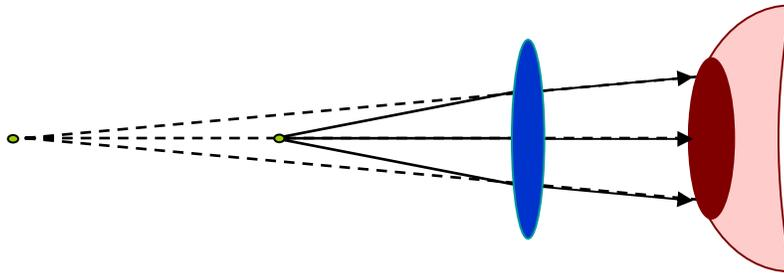
Now just to make the point even more forcefully, in all three situations below, the virtual image is in the same position although the actual object is in 3 different places.
