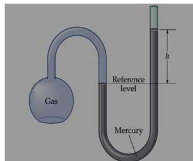
To find the temperature of a substance, the gas flask is placed in thermal contact with the substance. When the temperature is high, the pressure is large. From the graph of pressure versus temperature, you can easily read off the temperature. Note that we are using two fixed points, which we call  $0^{\circ}\text{C}$  and  $100^{\circ}\text{C}$ . This is called the Centigrade scale, and the two fixed points correspond to the freezing and boiling of water.
