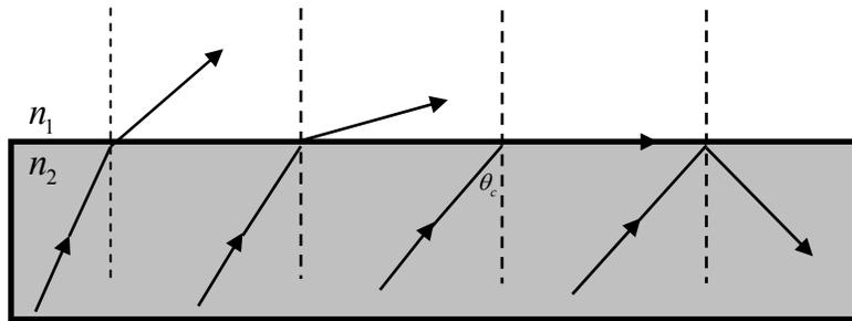
8. Fibre optic cables, which are now common everywhere, make use of the total internal reflection principle to carry light. Here is what a fibre optic cable looks like from inside:
