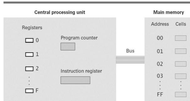
Figure 43: CPU and Main memory linkage using Bus
