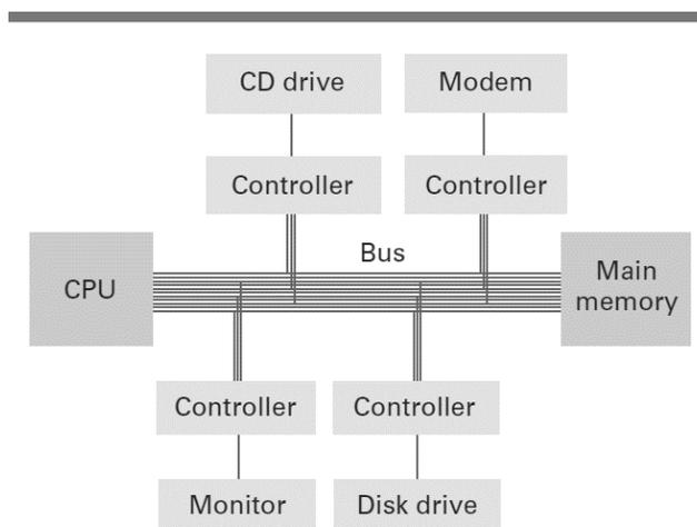
Figure 48: Controllers attached to a machine's bus
