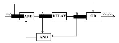
It is to be noted that in this sequential circuit, delay box plays an important role in introducing four states of the machine.
