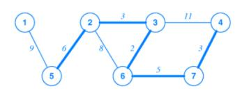
The shortest path in the figure from node 2 to node 6 is 2 to 3 and 3 to 6 as this path has the smallest weight so it is the shortest path.
