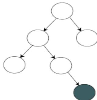
Though the original tree was balanced, more than one rotation is needed to restore balance following the insertion.
