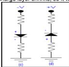
In **fig. c** the negative voltage has been applied to the anode of the diode through a resistance and cathode terminal of the diode is connected to the neutral terminal through resistance. Which will fulfill the condition of reversed biased.
