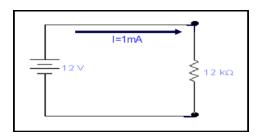
So the current flowing through all resistors by Ohm's law
