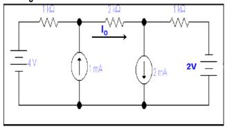
**Solution:** We want to calculate the **current I** $_{0}$ . The circuit can be redrawn as
