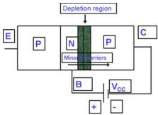
This fig shows the Collector-base junction where collector is made up of P-type material and Base is made up of N-type material. In the fig +ve terminal of the battery is connected to Base while –ve terminal is connected to the the Collector. Its mean this junction will go in to reverse-biased mode and depletion layer will be widened and the current will flow due to minority carriers.
