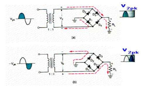
between the two diodes. When one is on( conducting), the other if off( non conducting), and vice versa. The bridge rectifier works basically in the same way. The main difference is that the bridge rectifier alternates conduction between two diodes pairs.
