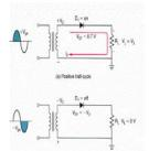
Therefore, all of V<sub>2</sub> is dropped across the diode in the rectifier.
