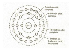
When there are many atoms closed in a copper wire, the outermost electrons are not sure from which atom they belong to.
