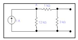
So the current flowing through series combination of  $1k\Omega$  and  $3k\Omega$  can be calculated as
