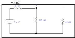
12kΩ is parallel with 4kΩ resistor so 12k||4k = (12 x4)/(12+4)
