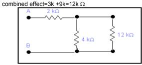
12k  $\Omega$  is in parallel with 4k  $\Omega$  so
