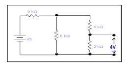
We want to calculate the source voltage. The voltage across  $2k\Omega$  resistor is 4V, so the current flowing through it will be
