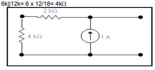
$2k\Omega$  resistor is in series with  $4k\Omega$  resistor so the total resistance will be
