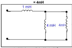
4mH is in parallel with 4mH So  $4mH||4mH = (4 \times 4)/(4 + 4)$ = 16/8 = 2 mH
