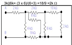
10k  $\Omega$  is in series with 2k  $\Omega$ , therefore, their combined effect =10k+2k=12k  $\Omega$
