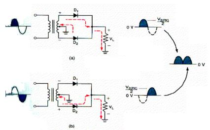
When the polarity of the input reverses,  $D_2$  is forward biased, and D1 is reverse biased. The direction of the current through the load will not change even though the polarity of the transformer secondary will. Thus another positive half cycle is produced across the load
