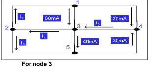
Now putting the value of  $I_5$  in equation of node 3  $I_4 -0.05 = 0.02$   $I_4 = 0.07 \text{ A}$
