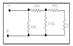
4k  $\Omega$  is in series with 8k  $\Omega$  so the combined effect=12k  $\Omega$
