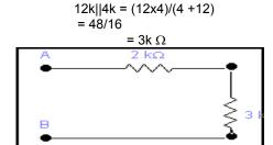
Now 2k  $\Omega$  is in series with 3k  $\Omega$  so R  $_{\mbox{AB}}$  = 2k +3k=5k  $\Omega$
