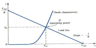
A sketch of the graphical construction is shown in the fig. The curve represents the exponential diode equation and the straight line represents the equation (2). Such a straight line is known as load line . The load line intersects the diode curve at point Q, which represents the operating point of the circuit. It co-ordinates gives values of  $I_D$  and  $V_D$
