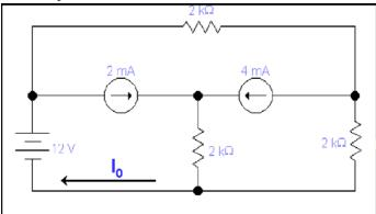
$\underline{\textbf{Solution:}} \ \ \text{We want to calculate the } \textbf{current I}_{\textbf{0}}. \\ \text{The circuit can be redrawn as}$
