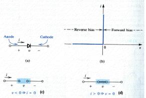
Fig a is diode circuit symbol , fig b is i-v characteristic fig c is equivalent circuit in the reverse direction and fig d is the equivalent circuit in the forward direction .
