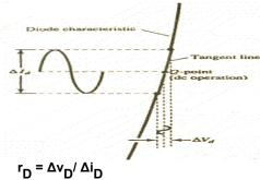
$\Delta$  shows a finite change in the quantity. The resistance in the vertical rise region is small, where as ac resistance is much larger at low current levels.
