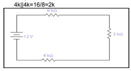
he resistors  $6k\Omega$ ,  $2k\Omega$  and  $4k\Omega$  are in series so they will be combined as=6k+2k+4k=12k  $\Omega_{\bullet}$
