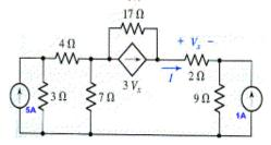
3 Ohms resistor is in parallel with 5A source. So it can be converted into a voltage source 15V.
