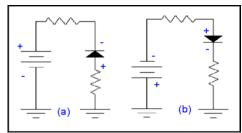
In **fig. a** the negative of the battery is connected to the anode through a resistor and positive terminal of the battery is connected the cathode therefore no current will flow and we can say that diode is not existing and it will act as an open circuit.
