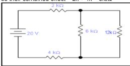
6k  $\Omega$  is in parallel with 12k  $\Omega$  so
