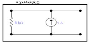
So the voltage drop across the equivalent  $6k\Omega$  resistor
