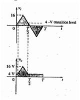
**EXAMPLE:** Consider in previous example the diode is silicon diode and draw its output.
