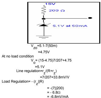
Example: Ghania is trying to design a shunt regulator, of about 20V, for her sister Azka's toy. Two kinds of zener diodes are available: 6.8V devices with  $r_z$  of 10 Ω and 5.1V devices with  $r_z$  of 30 Ω. For the
