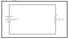
The current flowing through 40 ohm resistor by Ohm's law is I=V/R=40/40=1 A
