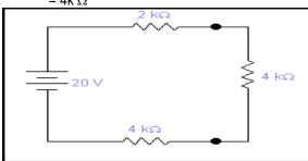
The resistors  $2k\Omega$ ,  $4k\Omega$  are in series so the combined effect will be =2k+4k+4k
