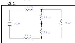
$4k\Omega$  is series with  $2k\Omega$  so their combined effect = 2k + 4k =  $6k\Omega_{\bullet}$
