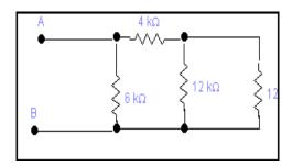
12k  $\Omega$  is in parallel with 12k  $\Omega$  so 12k||12k=(12 x 12)/(12+12)
