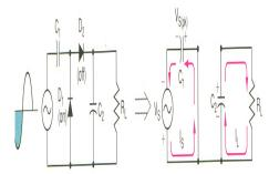
When the input polarity reverses, we have the circuit conditions show in the fig below. Since D1is off ,it is represented as an open in the equivalent circuit. Also , D2 (which is on ) is represented as a short. Using the equivalent circuit, it is easy to see that C1(which is charged to the peak value of Vs) and the source voltage now act as series –aiding voltage sources. Thus , C2 will charge to the sum of the series peak voltages.  $2V_{S(pk)}$ .
