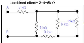
6k  $\Omega$  is in parallel with 6k  $\Omega$ , therefore,
