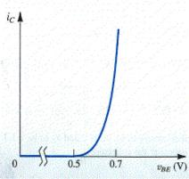
This curve has been drawn between the voltage across BEJ and the collector current. We can observe that the exponential rise in this collector current starts almost after 0.5 volts and saturated at 0.7 volts.
