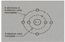
This outermost ring requires 8 electrons stability, except, when there is only one ring which require only 2 electrons for its stability.
