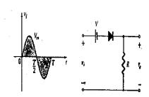
greater than V volts to turn the diode on. The negative region of the input signal is pressuring the diode into off region.
