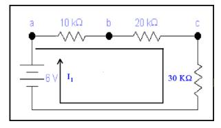
Let the current  $\mathbf{I_1}$  is flowing through the circuit. The **KVL equation** will be
