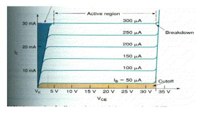
Along x-axis we are taking  $V_{CE}$  and along y-axis we are taking current collector current  $I_{C.}$
