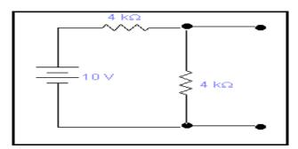
Now 4k is in parallel with 4k so we can Apply voltage division rule V= 4/8 x 10=5 volts
