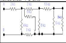
3k  $\Omega$  is in parallel with 6k  $\Omega$
