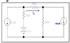
$\underline{\textbf{Solution:}} \ \ \text{We want to calculate the current I}_{0}. \ \text{To apply KVL the circuit can be}$
