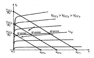
$\underline{\text{Example:}} \text{ Given a curve find V}_{\text{cc}}, \\ \text{R}_{\text{c}}, \\ \text{and R}_{\text{B}} \text{ for fixed bias circuit.}$
