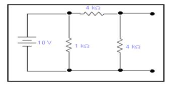
Now the voltage source is in parallel with the 1 k resistor so the voltage will be same.
