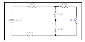
2k  $\Omega$  is in series with 2k  $\Omega$  so their combined effect =2k+2k=4k  $\Omega$
