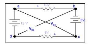
To calculate  $V_{\mbox{ac}}$ , the two paths will be acda and acba.
