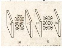
The work to be done in moving some electrons, as illustrated. Assume a charge of 1C can move three electrons. In Fig  $\bf a$  Then the charge of +3C can attract 9 electrons toward right. However, a charge of +1 C at the opposite side can attract 3 electrons towards left. The net result, then is that 6 electrons can be moved toward the right to the more positive charge.
