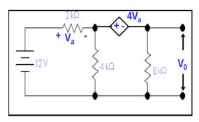
Solution: We want to calculate the voltage  $V_0$ . The circuit can be redrawn as
