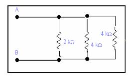
4k  $\Omega$  is parallel with 4k  $\Omega$  so 4k||4k = (4 x 4)/(4 +4) =16/8 = 2k  $\Omega$
