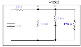
12k $\Omega$  is parallel with 6k $\Omega$  resistor so 12k||6k = (12 x 6)/18 = 72/18
