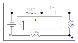
$\underline{\textbf{Solution:}} \quad \text{We want to calculate the voltage } \textbf{V}_{\textbf{bd}}. \\ \text{First we will have to calculate the voltage across 40k resistor.}$
