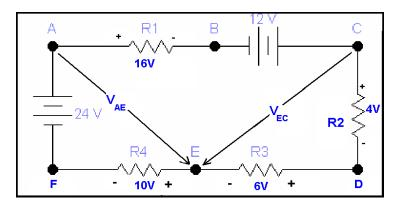
Since points A and E as well as E and C are not physically close, we use the arrow notation. Our approach to determining the unknown voltage is to apply KVL with the unknown voltage in the closed path, therefore to  $V_{AE}$  we will use the path **AEFA** or **ABCDEA**. The equation for two paths in which  $V_{AE}$  is the only known are
