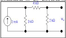
2mA source is in parallel with 3k source so it can be converted into a voltage V=2 x3 = 6volts (by Ohm's Law)
