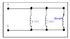
**Solution:** 6mH is in parallel with 3mH so
