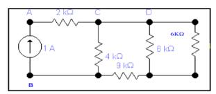
At point c the current should divide into two parts but due to short circuit between c and D whole current will come at point D.
