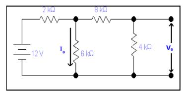
$\underline{\textbf{Solution:}} \quad \text{We want to calculate the current I}_{\pmb{0}} \text{ and the voltage V}_{\pmb{0}}. \text{ The circuit can}$
