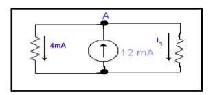
By KCL the equation for node A -12mA + 4mA + I =0
