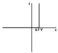
Figure C\_a: Practical diode model.
