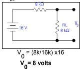
$\underline{\textbf{Example:}}$  Calculate the voltage  $\mathbf{V}_{\mathbf{O}}$  by using Thevenin's theorem .
