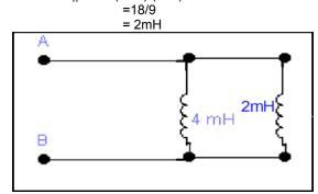
2mH is in parallel with 4mH, therefore, 2mH||4mH =  $(2 \times 4)/(2+4)$ = 8/6=1.33mH
