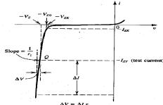
In case of zener diode the differential voltage and current in the zener region of the characteristic curve is given by
