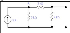
The current is dividing between  $3k\Omega$  and series combination of  $2k\Omega$  and  $4k\Omega$  so by current division rule I = (3k/(3k+6k))x (-2)
