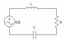
If  $V_L$ ,  $V_R$  and  $V_c$  denote the voltage drop across the inductor, resistor and capacitor respectively. Then
