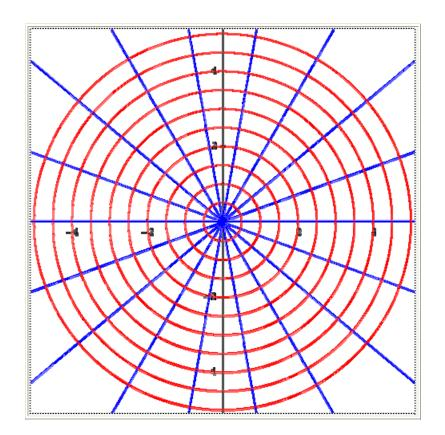
Clearly whenever one line intersects one circle, the tangent line to the circle (at the point of intersection) and the line are perpendicular i.e. orthogonal to each other. We say that the two families of curves are orthogonal at the point of intersection.
