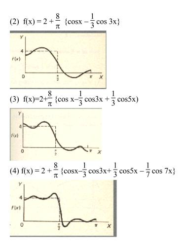
As the number of terms is increased, the graph gradually approaches the shape of the original square waveform. The ripples increase in number and decrease in amplitude, but a perfectly square waveform is unattainable in practice. For practical purpose, the first few terms normally suffice to give an accuracy of acceptable level.
