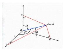
The angles which a line makes with positive x,y and z-axis are known as Direction Angles. In the above figure the blue line has direction angles as  $\alpha$ , and which are the angles which blue line makes with x,y and z-axis respectively.
