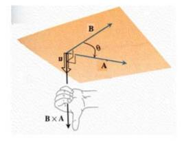
We start with two nonzero nonparallel vectors  $\mathbf{A}$  and  $\mathbf{B}$ . We select a unit vector  $\mathbf{n}$ Perpendicular to the plane by the **right handed rule**. This means we choose  $\mathbf{n}$  to be the unit vector that points the way your right thumb points when your fingers curl through the angle 0 from  $\mathbf{A}$  to  $\mathbf{B}$ .
