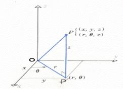
In the figure we have the projection of the point P in the xy-Plane and write its position in plane polar coordinates and also represent the angle  $\theta$  now from that projection we draw perpendicular to both of the axis and using the trigonometric ratios find out the following relations.
