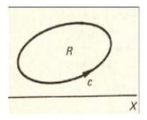
That is, a double integral over the plane region R can be transformed into a line integral over the boundary c of the region - and the action is reversible.
