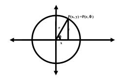
From above diagram and remembering the trigonometric ratios we can write  $x = r \cos \theta$ ,  $y = r \sin \theta$ . Now squaring these two equations and adding we get,
