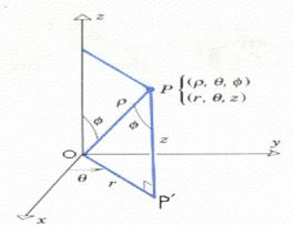
First we will find the relation between Planes polar to spherical, from the above figure you can easily see that from the two right angled triangles we have the following relations.
