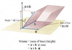
By treating the planes of b and c and of c and a as he base planes of the parallelepiped determined by a, b and c
